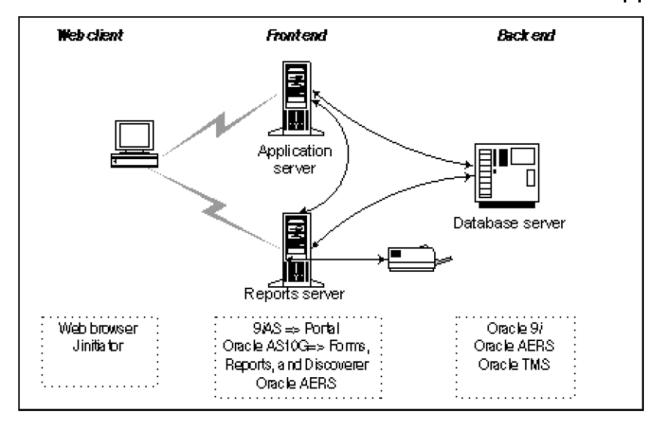
Oracle AERS consists of a back end Oracle 9i RDBMS, middle-tier computers, and Web clients. The middle-tier computers are the 9iAS Application Server and the AS10g Reports and Forms Servers. We no longer support client/server deployments.
