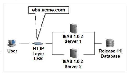
In this configuration, end-users navigate to a specific *Web Entry Point* that represents your E-Business Suite's domain name. An HTTP Layer load-balancer routes all subsequent traffic for a specific user to a specific Web Node.
